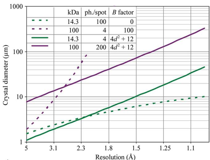
**Figure 5** Resolution-dependence of the minimum required crystal size. All plotted calculations used  $V_M = 2.4 \text{ \AA}^3 \text{ Da}^{-1}$  and 1 Å radiation. The Wilson *B* factor strongly affects the curvature of the plot of the required crystal size for a given number of photons, but applying the empirical formula shown serendipitously simplifies this analysis, as described in the text.
